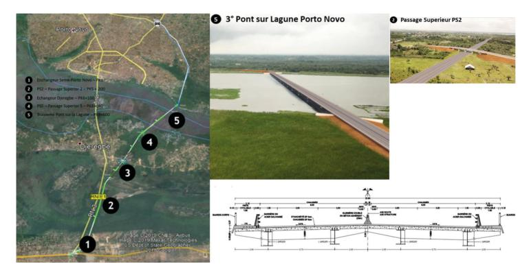
Preliminary Project of a carriageway connection between the Seme crossroads and Porto-Novo with the construction of a bridge over the lagoon and the 2X2 lane connection to the Boulevard du Cinquentenaire
