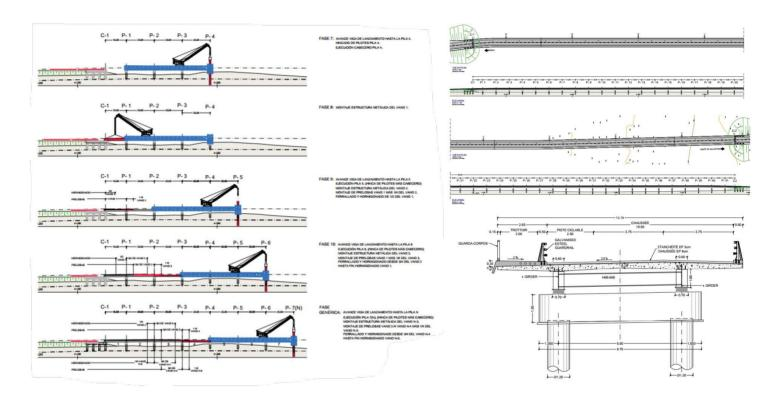
Single carriageway with one lane in each direction and a ciclepath, including 5 composite steel-concrete girder, with a máximum lengh of 830 m
